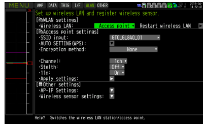
Access point settings
